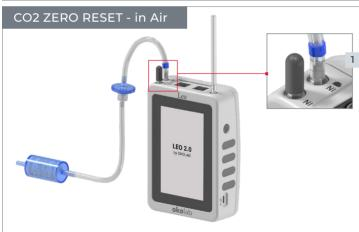
1 Connect the **blue labeled end** of SODA LIME KIT to LEO 2.0 gas inlet port labeled with icon  $\center{l}$  and put the cap on the other gas inlet port.
